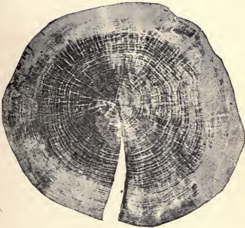
FIG. 26.—Photograph of the transverse section of a log of oak, about one-sixth natural size. The cortex and bark are removed, and the outline is bounded by the cambium. The pith appears as a mere dot in the centre; the medullary rays radiate from this, and the annual rings (about forty in number) are arranged concentrically around it. A large crack has formed along the plane of a medullary ray as the section dried. (Müller.)
